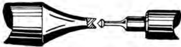
Lump left at end of pivot, due to excessively large back centre
